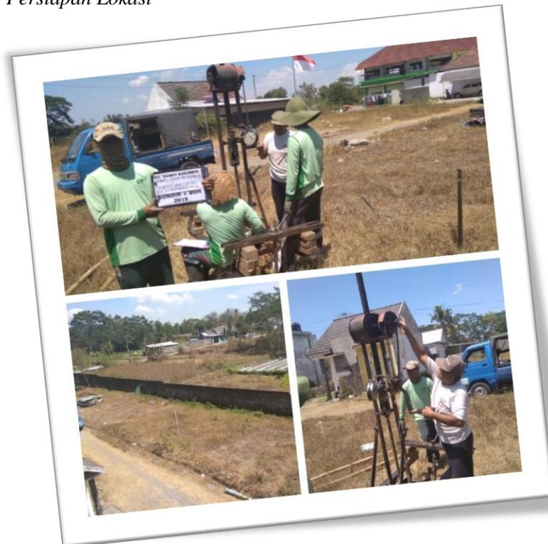
*Gambar 2 Proses Sondir*
